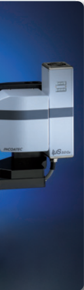
D8 QUEST compact configuration with: - \mu S 3.0 source - HELIOS MX optics - KAPPA goniometer - PHOTON II detector
